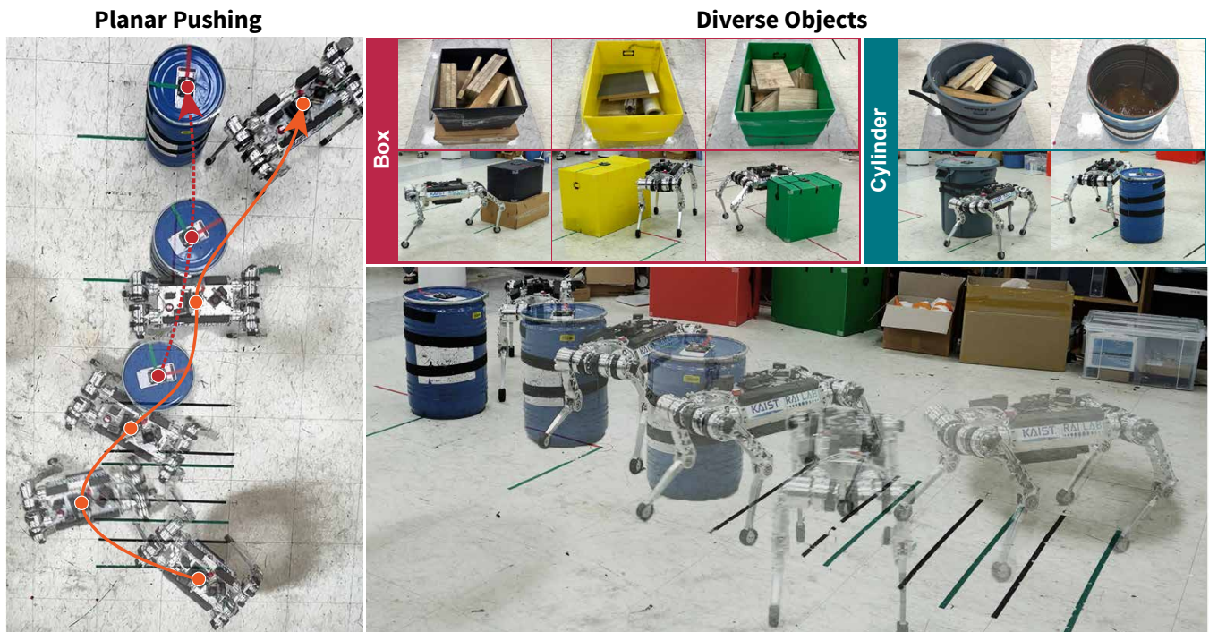
Fig. 1: Whole-body manipulation for planar pushing: The proposed system enables a quadrupedal robot, weighing 27\text{ kg} , to manipulate its entire body to re-pose an object in a 2D plane. Our system does not require the object’s physical properties or dimensions but achieves an implicit understanding of the object’s properties through real-time interactions. Experiments were conducted on a total of five different objects with diverse properties. The robot can adapt even when the object’s physical properties change dynamically, such as when dealing with a 19.2\text{ kg} water-filled drum that is approximately 70\% of the robot’s weight.
